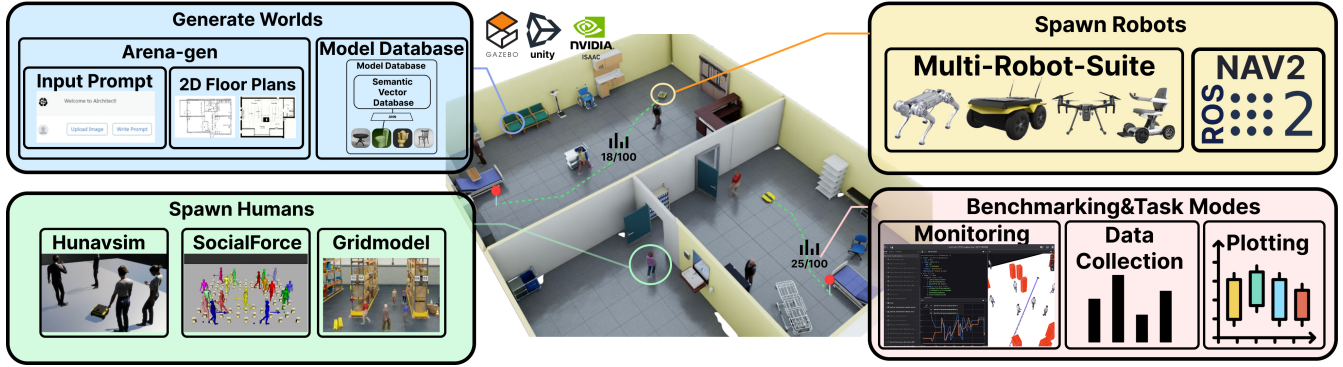
Fig. 2: Data flow of the Generation Stage and the Population Stage . The Generation Stage combines multiple SotA technologies to process text inputs into a floor plan image and room asset locations. 3DSGs are used as an intermediate data structure to divide the problem into a text transformation task solvable by an LLM, and a graph transformation task solvable by a spatial GNN. The Population Stage populates the floor plan’s asset zones with 3D models by employing the Asset Placer . A pre-built semantic vector Model Database is queried for a related model, which is arranged into the zone by a Fitter algorithm. After a final post-processing step, the end result is a finished environment consisting of 3D walls and models.
