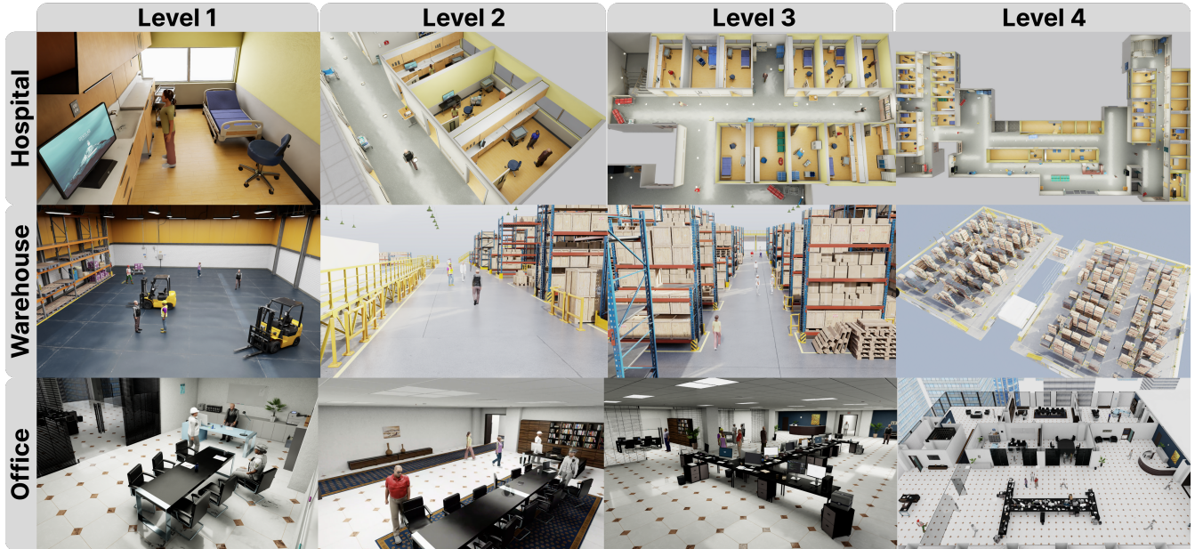
Fig. 9: Example worlds generated using the Arena-Gen module for benchmarking and competition purposes. The worlds were generated using the text "generate 4 difficulty levels of a [hospital, residential, office] environment". The assets are automatically taken from the arena model database and pedestrians spawned with HuNavSim. Notably, a large variety of worlds for each environment type and level can be generated, e.g. 500 environments of hospital level 2. This feature aids quantitative benchmarking and in training new models. Users can also customize room layouts, pedestrian interactions with each other, asset placements, and specific situations using the Arena Architect GUI (shown in the supplementary video).
